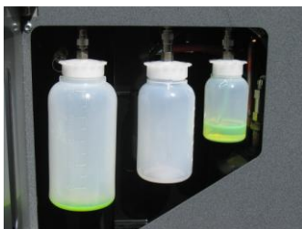
Waste, new oil & dye injection Totally automatic with presets
