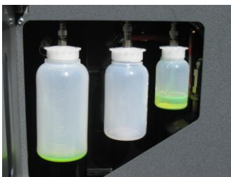
Waste, new oil & dye injection Totally automatic with presets
