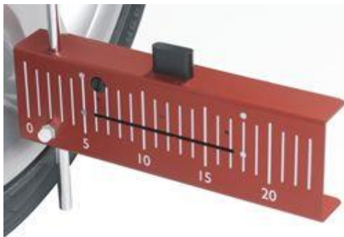
Rear scale with LED's showing steering wheel position
